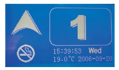
Information display via LCD can be provided on the car operating panel (COP) or at the lift lobby above the lift entrance or the transom panel (in lieu of the standard dot matrix indicator).
